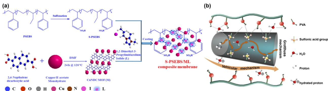
**Fig. 9** (a) Schematic representation for preparation of S-PSEBS/ML composite membrane. Reproduced with permission from ref. 83, Copyright 2022, American Chemical Society. (b) The possible proton transport pathways of CL-PVA/Cu-MOF-15. Reproduced with permission from ref. 84, Copyright 2023, Elsevier.
