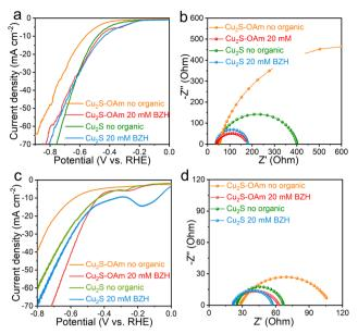
Fig. 3 (a) LSV curves and (b) Nyquist plots at -0.7 V vs. RHE of Cu<sub>2</sub>S-OAm and Cu<sub>2</sub>S in 1 M sodium acetate-acetic acid electrolyte (pH = 5.2) with and without BZH at room temperature; (c) LSV curves and (d) Nyquist plot at -0.7 V vs. RHE of Cu<sub>2</sub>S-OAm and Cu<sub>2</sub>S in 1 M potassium carbonatepotassium bicarbonate electrolyte (pH = 9) with or without BZH at room temperature
