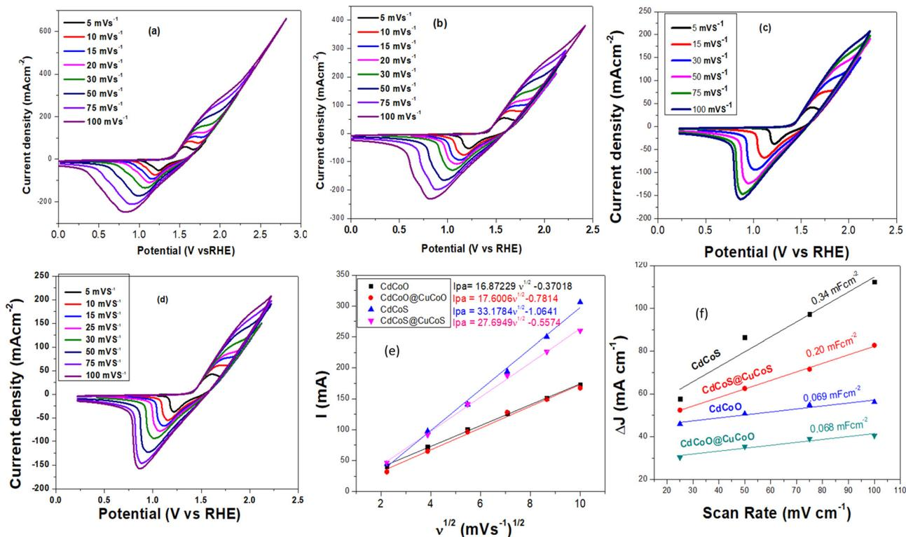
Fig. 5 Cyclic voltammograms (CV) of the catalysts (a) CdCoS, (b) CdCoS@CuCoS, (c) CdCoO, and (d) CdCoO@CuCoO. The plots are between the anodic peak current ( $I_{\text{pa}}$ ) of cyclic voltammograms in 1.0 M KOH and the square root of the scan rates ( $v^{1/2}$ ) for all the as-synthesized catalysts.
