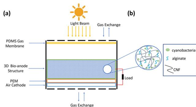
**Fig. 1** Schematic of a 3D hydrogel-based bio-anode embedded BPV cell unit for energy harvesting. (a) Schematic of 3D hydrogel-based bio-anode embedded BPV cell unit (b) components of the 3D hydrogel-based bio-anode structure.
