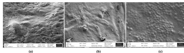
**Fig. 8** Results of SEM analysis for 3D bioanode structure (a) reference, only sodium alginate, and CNF hydrogels. Scale bar – 200 nm. (b) *Synechocystis* sp. PCC 6803 seeded bioanode structure, scale bar – 20  $\mu\text{m}$ . (c) *Synechocystis* sp. PCC 6803 seeded bioanode structure, scale bar – 2  $\mu\text{m}$ .
