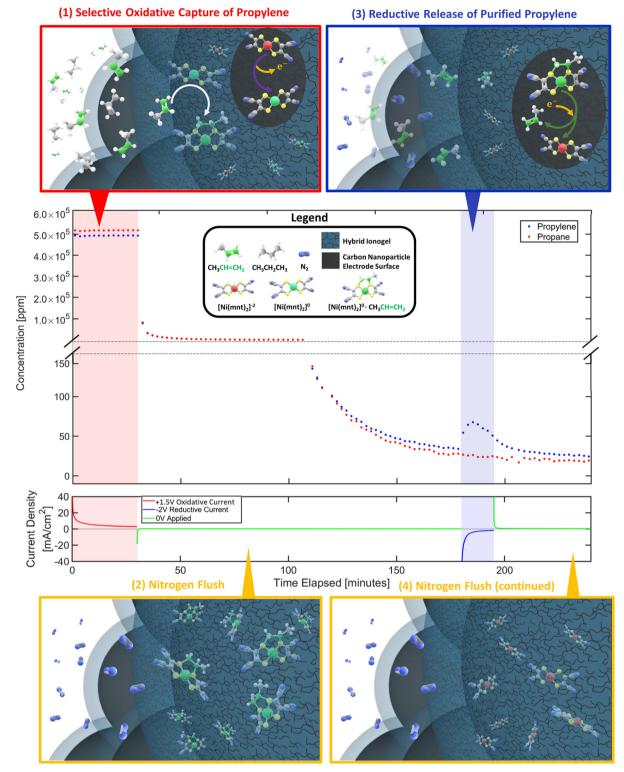
Fig. 2 Propylene gas separation performance was quantified for each MEA sample by keeping periodic GC measurements of the output gas stream's composition for a duration of 4 hours per experimental run cycle, a sample experimental cycle of which is demonstrated above. Each cycle consists of 4 distinct phases: (1) selective oxidative capture of olefin, (2) nitrogen flush, (3) reductive release of purified olefin, (4) final nitrogen flush.
