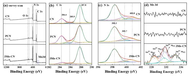
Fig. 3 XPS survey scan (a), and high resolution C 1s (b), N 1s (c) and Mo 3d (d) spectra of CN, PCN and 3Mo-CN.
