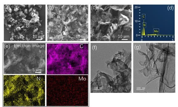
Fig. 1 SEM images of CN (a), PCN (b), and 3Mo-CN (c). EDS spectrum (d) and electron image and corresponding EDS element mapping (e) of 3Mo-CN. TEM images of PCN (f) and 3Mo-CN (q).
