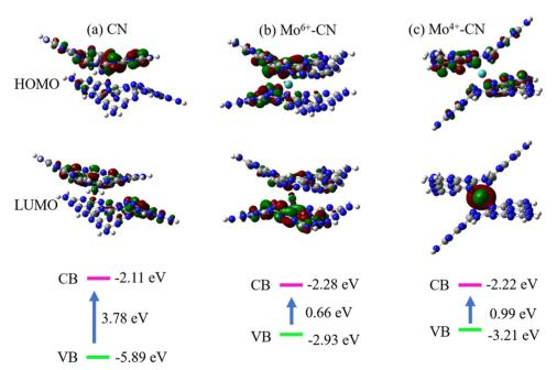
Fig. 8 HOMO, LUMO, and band gap of CN (a),  $Mo^{6+}$  – CN (b) and  $Mo^{4+}$  – CN (c). The iso-surface value is set at 0.03 e bohr<sup>-3</sup>. Denotation: C atom – gray, N atom – dark blue.
