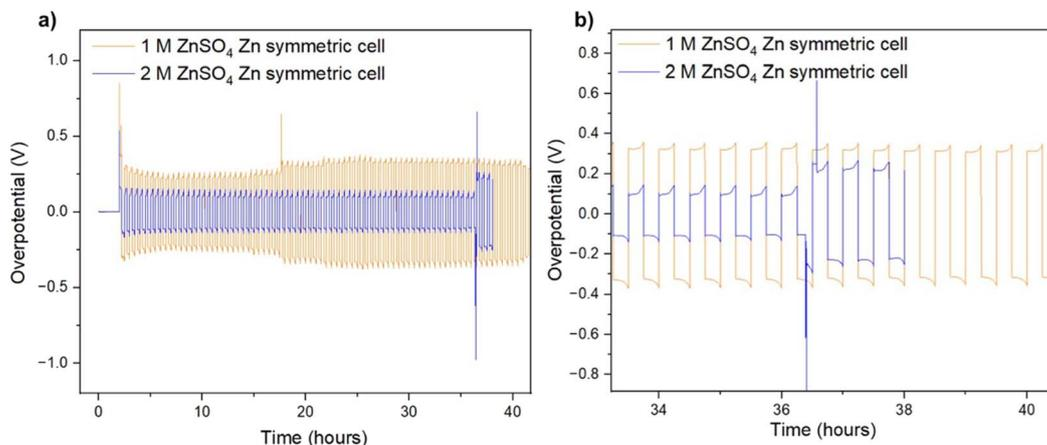
Fig. 8 (a) Voltage trace ( $E$  vs.  $t$ ) of successive galvanostatic cycling of a total of 2.75 mA h cm<sup>-2</sup> of zinc at 11 mA cm<sup>-2</sup> (4C) in zinc symmetric cell with 2 M ZnSO<sub>4</sub> aqueous electrolyte, glass fibre separator. (b) Magnification of voltage trace ( $E$  vs.  $t$ ) at the soft short formation.
