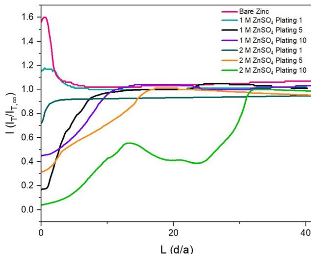
Fig. 3 Probe approach curves measured at various stages of cycling at  $1.7 \text{ mA cm}^{-2}$ . Measurements were recorded after the first, fifth, and tenth plating for zinc-metal anodes in 1 M and 2 M  $\text{ZnSO}_4$ . An increase in tip current beyond  $l = 1$  denotes positive feedback, and a decrease in tip current below  $l = 1$  denotes negative feedback. A charge of  $1.7 \text{ mA h cm}^{-2}$  ( $4 \text{ mg cm}^{-2}$  zinc) was passed per plating/stripping cycle.
