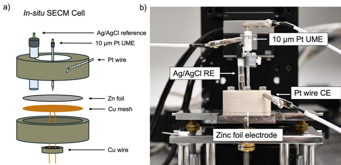
Fig. 2 (a) Schematic of the *in situ* 4-electrode scanning electrochemical microscope cell using a zinc foil working electrode, a 10 μm platinum ultramicroelectrode, a Pt wire counter electrode and a saturated Ag/AgCl reference electrode. (b) A photo of the *in situ* scanning electrochemical microscopy cell used with the CH Instruments 920C SECM instrument.
