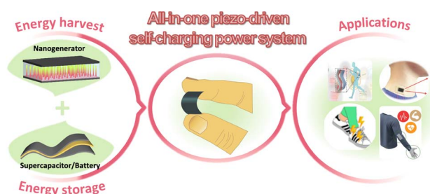
Fig. 1 Schematic diagram of the all-in-one piezo-driven self-charging power system. Reproduced from ref. 23 with permission from Elsevier, copyright 2018; reproduced from ref. 24 with permission from Elsevier, copyright 2019; reproduced from ref. 25 with permission from Wiley-VCH GmbH, copyright 2017; reproduced from ref. 26 with permission from American Chemical Society, copyright 2019.
