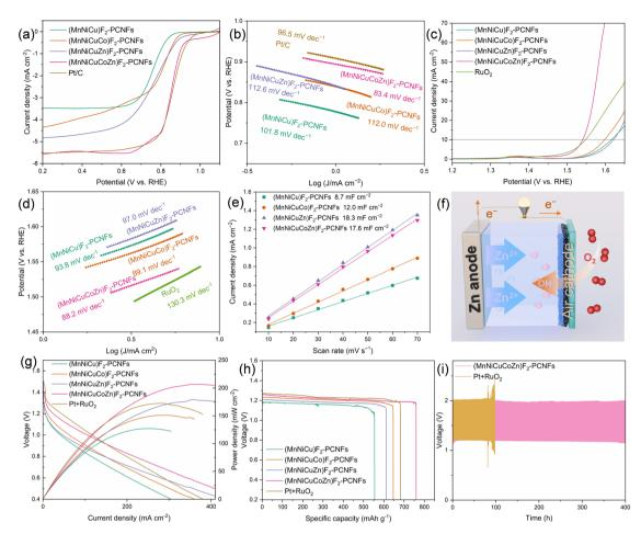
Fig. 5 (a) Polarization curves and (b) corresponding Tafel slopes for the ORR. (c) OER performance and (d) corresponding Tafel slopes. (e)  $C_{\rm dl}$ fitting curves. (f) Schematic of a ZAB, (g) discharge polarization curves and corresponding power density curves, (h) continuous discharge curves, and (i) charge-discharge cycles.
