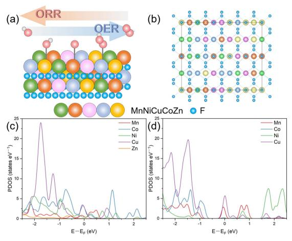
Fig. 6 The adsorption state model and reaction process schematic diagram of (a) the OER/ORR process and (b) the structure model of (MnNiCuCoZn)F<sub>2</sub>. Partial Density of States (PDOS) diagrams for (c) (MnNiCuCoZn)F<sub>2</sub> and (d) (MnNiCuCo)F<sub>2</sub>.
