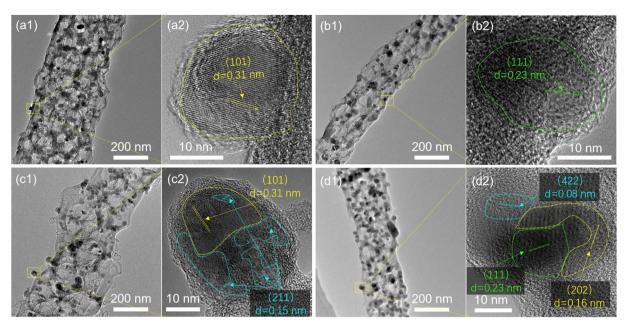
Fig. 2 The high-resolution transmission electron micrographs (HR-TEM) of (a1 and a2) (MnNiCu) $F_2$ -PCNFs, (b1 and b2) (MnNiCuCo) $F_2$ -PCNFs, (c1 and c2) (MnNiCuZn) $F_2$ -PCNFs, and (d1 and d2) (MnNiCuCoZn) $F_2$ -PCNFs.
