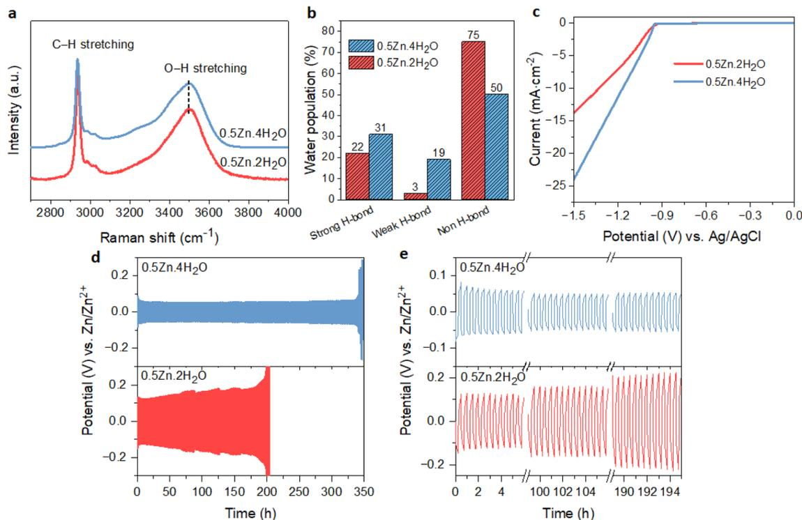
Fig. 6 Solvation structure and electrochemical stability of the Zn anode in 0.5Zn·4H<sub>2</sub>O electrolyte compared to concentrated 0.5Zn·2H<sub>2</sub>O. (a) Raman spectra in the water region. (b) The corresponding water population percentages. (c) LSV curves on a Ti substrate (d) Zn plating/stripping at 2 mA cm<sup>-2</sup> and 0.5 mA h cm<sup>-2</sup> in Zn||Zn symmetric cells and (e) the corresponding potential profiles.
