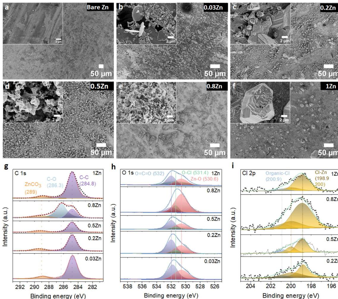
Fig. 5 Morphology evolution and surface composition of Zn electrodes after 20 cycles of Zn plating/stripping in different WISEs at  $1 \text{ mA cm}^{-2}$  and  $0.5 \text{ mA h cm}^{-2}$ . SEM images of (a) bare Zn and a cycled Zn anode in (b) 0.03, (c) 0.2, (d) 0.5, (e) 0.8, and (f) 1Zn electrolytes. The corresponding (g) C 1s, (h) O 1s, and (i) Cl 2p XPS spectra.
