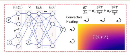
Fig. 2 Application of ML in the prediction of temperature using spacial and temporal parameters as independent variables in transient convection of a porous medium, Zobeiry and Humfeld,<sup>47</sup> reproduced with permission from Elsevier.
