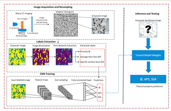
Fig. 5 A flow work to predict porous properties of porosity ( $\phi$ ), specific surface area (SSA), and average pore size (APS) by a CNN using image acquisition, visually/experimentally input parameter extraction, and construction of a tuned neural network for prediction, Alqahtani *et al.*,<sup>97</sup> reproduced with permission from Elsevier.
