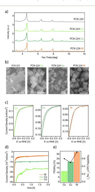
Fig. 3 (a) Powder diffraction of PCN-224 and the metalated PCN-224-M derivatives. (b) SEM images of the isolated solids showing the formation of cube-like crystals with varying sizes. (c) CV at 50 mV s $^{-1}$ for each PCN-224-M framework under an Ar (gray) and N<sub>2</sub> atmosphere (color). (d) CA at -0.04 V vs. RHE for the same materials and (e) comparison of faradaic efficiencies and yields for ammonia generation.
