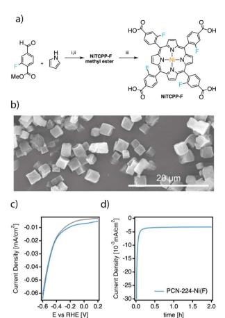
Fig. 5 (a) Experimental procedure for the synthesis of the NiTCCP-F linker: (i) DCM, pyrrole, BF<sub>3</sub>·OEt<sub>2</sub>, stirring 2 h, then add p-chloranil, reflux for 2 h, (ii) Ni<sup>2+</sup>, DMF, reflux overnight, and (iii) MeOH, THF and KOH, reflux overnight and wash with acetic acid. (b) SEM micrograph of PCN-224-Ni(F) crystals. (c) CV at 50 mV s<sup>-1</sup> under an Ar (gray) and  $N_2$  atmosphere (color) and (d) CA at -0.04 V vs. RHE of the fluorinated framework
