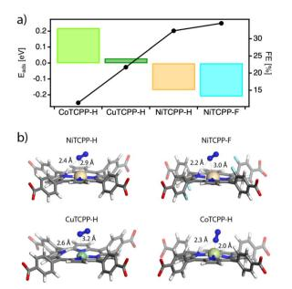
Fig. 6 (a) DFT adsorption energy ( $E_{ads}$ ) calculated for MTCPP-X (M=Ni, Co, Cu and X=H, F) cluster models according to the Tafel-Volmer mechanism (left axis) and correlation with the experimental FE values (right axis). (b) Calculated models showing the adsorption of  $N_2$  molecules (in blue) to the catalytic site and distances with the protonated porphyrin in all cases studied.
