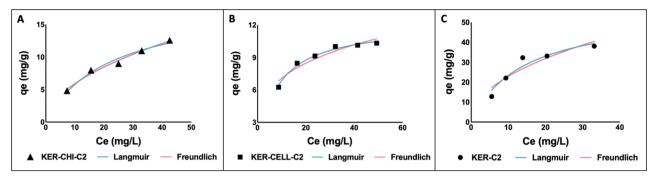
Fig. 4 Experimental absorption isotherms of RB4 at pH 2.0 using different keratin-based films: KER-CHI-C2 (A); KER-CELL-C2 (B); and KER-C2 film (C).
