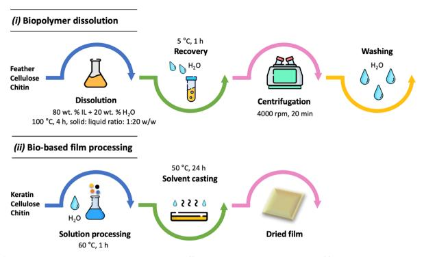
Fig. 1 Schematic representation of the biopolymer dissolution (i) and the keratin-based film processing (ii) proposed in this work.
