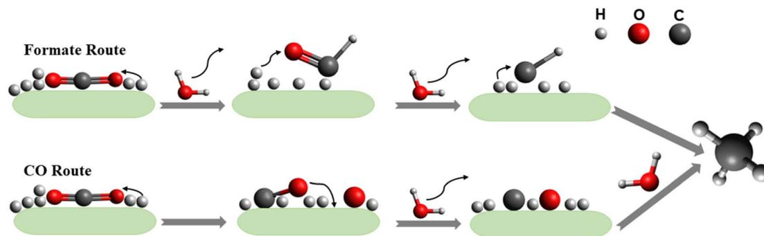
Fig. 7 General routes for CO<sub>2</sub> hydrogenation through the CO route and formate route.
