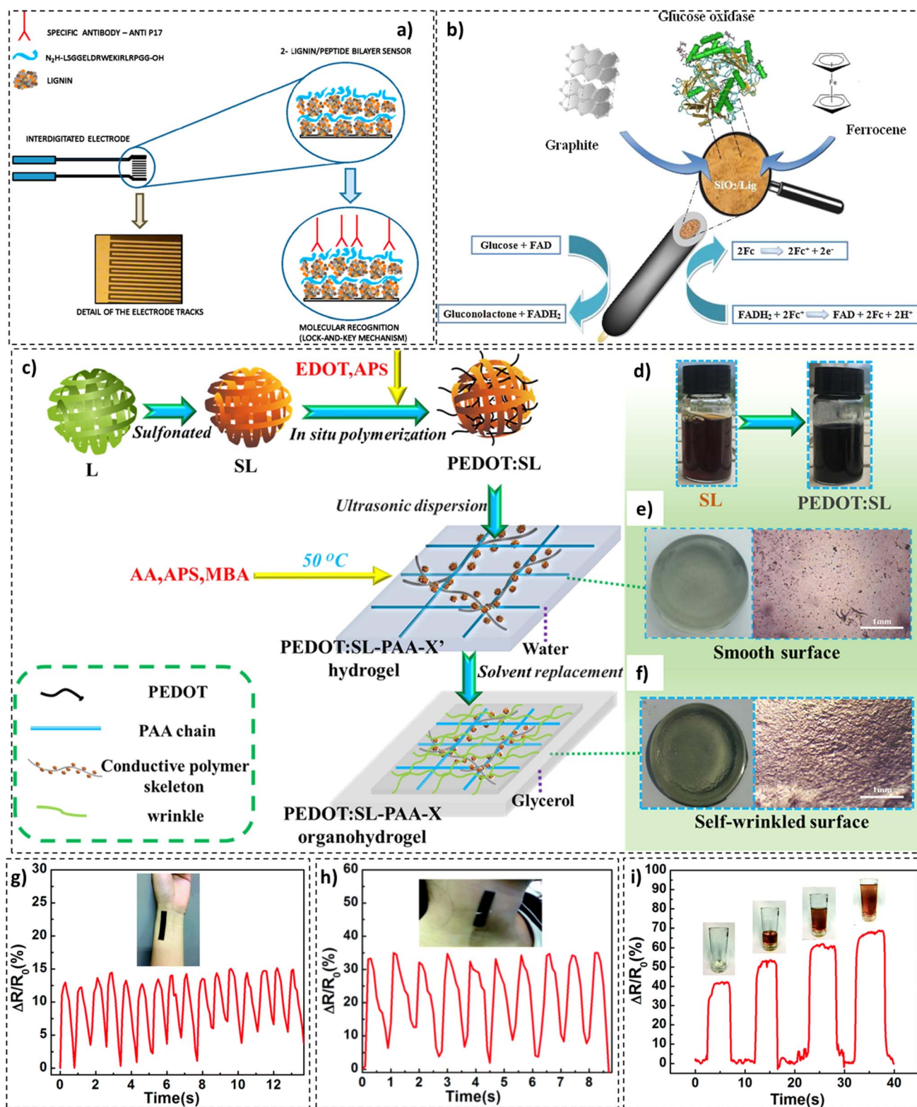
Fig. 13 (a) Electrical impedance spectroscopy (EIS) based immunosensors (reproduced from ref. 226 with permission from Elsevier, copyright 2015), (b) functional GOx/silica/lignin system based carbon paste electrode (reproduced from ref. 229 with permission from Elsevier, copyright 2018), (c) synthesis of PEDOT:SL-PAA organohydrogel, (d) color change during synthesis, (e) morphology of PEDOT:SL-PAA hydrogel, and (f) morphology of a PEDOT:SL-PAA organohydrogel composite based wearable device: (reproduced from ref. 230 with permission from Elsevier, copyright 2019) CL/PDMS (g) for wrist pulse measurement, (h) for neck pulse measurement, and (i) power measurement in picking up a cup (reproduced from ref. 231 with permission from RSC, copyright 2018).
