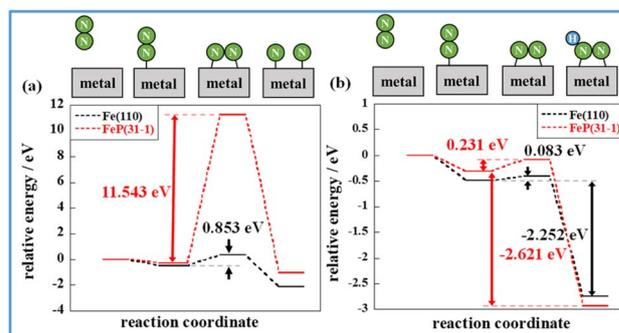
Fig. 9 Energy diagram of  $N_2$  dissociation (a) and  $N_2H$  formation (b) on Fe(110) and FeP(31–1). Activation energy for  $N_2$  dissociation in the absence of an electric field corresponds to the energy difference between the second state and the third state in (a).  $N_2H$  production energy in an electric field corresponds to the energy difference between the second state and the fourth state in (b).
