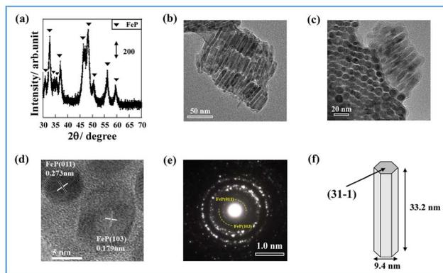
Fig. 1 Characterization of Fe phosphide: (a) XRD measurement, (b) TEM image (side view), (c) TEM image (bottom view), (d) high-resolution TEM image, (e) electron diffraction image for selected area, and (f) illustrated structure of Fe phosphide.
