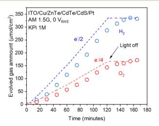
Fig. 10 Hydrogen and oxygen evolution from the ITO/Cu/ZnTe/CdTe/CdS/Pt (RTA) photocathode under simulated sunlight in a three-electrode configuration with an applied potential of 0  $V_{RHE}$ . The expected amounts of hydrogen and oxygen (denoted as  $e^-/2$  and  $e^-/4$ , respectively) as calculated from the observed photocurrent are shown as dashed lines. A 1 M aqueous KPi solution with pH adjusted to 6.5 with KOH was used as the electrolyte.
