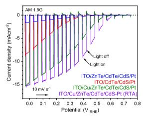
Fig. 5 Current-potential curves for ITO/CdTe/CdS/Pt, ITO/ZnTe/CdTe/CdS/Pt, ITO/Cu/ZnTe/CdTe/CdS/Pt, and ITO/Cu/ZnTe/CdTe/CdS/Pt (RTA) under chopped simulated sunlight. 1 M aqueous KPi solution with pH adjusted to 6.5 was used as an electrolyte. The applied potential was swept at +10 mV s $^{-1}$ .
