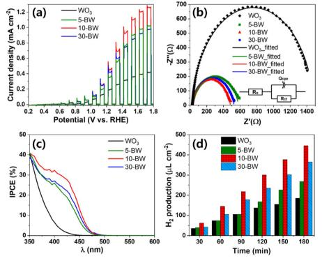
Fig. 4 Photoelectrochemical performances of the WO<sub>3</sub> nanocorals and BiVO<sub>4</sub>/WO<sub>3</sub> photoanodes of 5-BW, 10-BW, and 30-BW: (a) photocurrent densities by linear sweep voltammetry, (b) Nyquist plots and equivalent circuits, (c) PEC H2 production diagram as a function of time, and (d) IPCE spectra.
