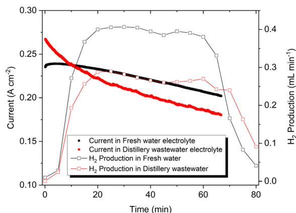
Fig. 6 H<sub>2</sub> generation of Ni<sub>2</sub>Se<sub>3</sub>/SS electrodes using fresh water (black) and distillery wastewater based electrolyte (red). Note that the concentration of electrolytes was 1.0 M NaOH.
