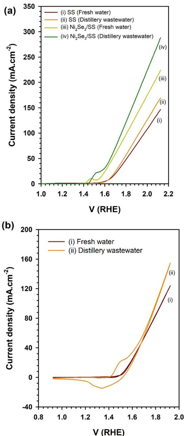
Fig. 3 (a) Linear sweep voltammogram results of stainless steel and Ni<sub>2</sub>Se<sub>3</sub> nanoparticles coated stainless steel substrates in freshwater and distillery wastewater electrolyte. (b) CV of Ni<sub>2</sub>Se<sub>3</sub>/SS anode in freshwater and distillery wastewater-based electrolyte. Note that the concentration of the electrolyte was 1 M NaOH.
