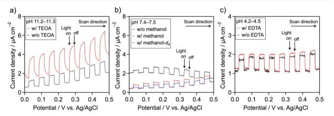
Fig. 2 Current–potential curves for Pt/meso-PCN/FTO electrodes under an Ar atmosphere and under irradiation with chopped visible light ( $\lambda$  > 400 nm), as recorded in aqueous Na<sub>2</sub>SO<sub>4</sub> (0.1 M) containing different additives: (a) TEOA, (b) methanol and (c) EDTA. Scan rate: 10 mV s<sup>-1</sup>. Note: w/and w/o in the figure indicate with and without, respectively
