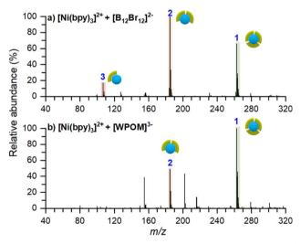
Fig. 6 Ex situ MS of surfaces prepared by co-depositing  $[Ni(bpy)_3]^{2+}$  with (a)  $[B_{12}Br_{12}]^{2-}$ , and (b)  $[WPOM]^{3-}$ . Both surfaces show an increased abundance of  $[Ni(bpy)_3]^{2+}$  and only minor products of dissociation.
