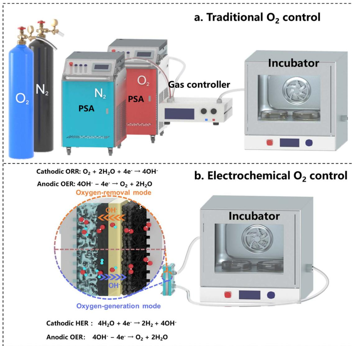
Fig. 4 Working mechanisms of different O<sub>2</sub>-control methods: (a) traditional O<sub>2</sub>-control method, and (b) electrochemical O<sub>2</sub>-control method.
