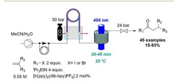
Scheme 3 Carbonylative hydroacylation of styrenes exploiting photochemical flow conditions.
