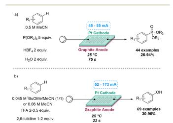
Scheme 11 Flow-based C-H phosphorylation and hydroxylation reactions exploiting electrochemistry.
