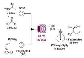
Scheme 13 Synthesis of homoallyl alcohols in flow mode.
