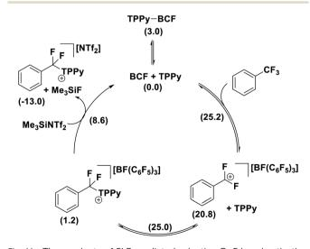
Fig. 11 The products of FLP mediated selective C-F bond activation are in equilibrium with the starting materials and require a fluoride sequestration agent to facilitate catalysis. Free energies in kcal mol<sup>-1</sup> given in parentheses.
