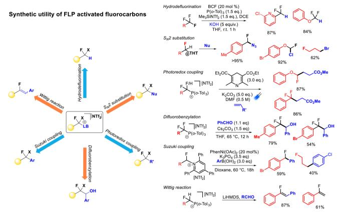
Fig. 12 A large number of functionalization reactions are possible post C-F bond activation. Judicious choice of Lewis base allows for specific functionalization. Thus far, formal hydrodefluorination, nucleophilic substitution, photoredox alkylation, nucleophilic transfer, Suzuki-Miyaura coupling and Wittig olefination have been demonstrated as post-activation functionalisations.
