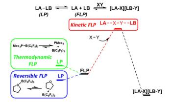
Fig. 7 Thermodynamic FLP exhibit an FLP ground state. This provides a thermodynamic platform to enhance reactivity. Kinetic FLP cooperate synergistically to activate bonds through concerted transition states involving both the Lewis acid and Lewis base. LB = Lewis base, LA = Lewis acid, LP = Lewis pair.
