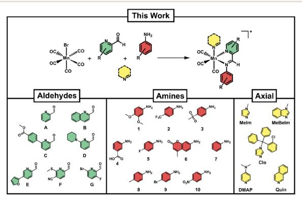
Fig. 2 General reaction scheme of the combinatorial synthesis of manganese tricarbonyl Schiff-base complexes and overview of chemical building blocks selected for the synthesis of 420 novel complexes (all 70 possible Schiff-base complexes where also synthesised without the addition of the N-donor axial ligand, likely leading to the coordination of a solvent molecule).
