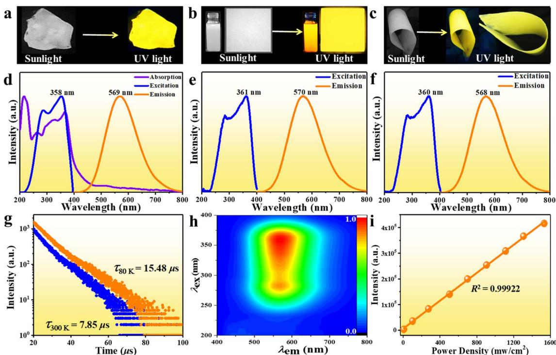
Fig. 2 PL characterization of  $(\text{Im-BDMPA})\text{In}_{0.78}\text{Sb}_{0.22}\text{Cl}_6 \cdot \text{H}_2\text{O}$ : (a–c) photo images of bulk crystals, microparticles, the deposited thin film and the flexible composite film under sunlight and 365 nm UV light; (d–f) absorption, excitation and emission spectra of bulk crystals, microparticles and flexible composite; (g) PL decay curves at 300 K and 80 K; (h) 3D consecutive PL map; (i) power density dependent PL emission intensity.
