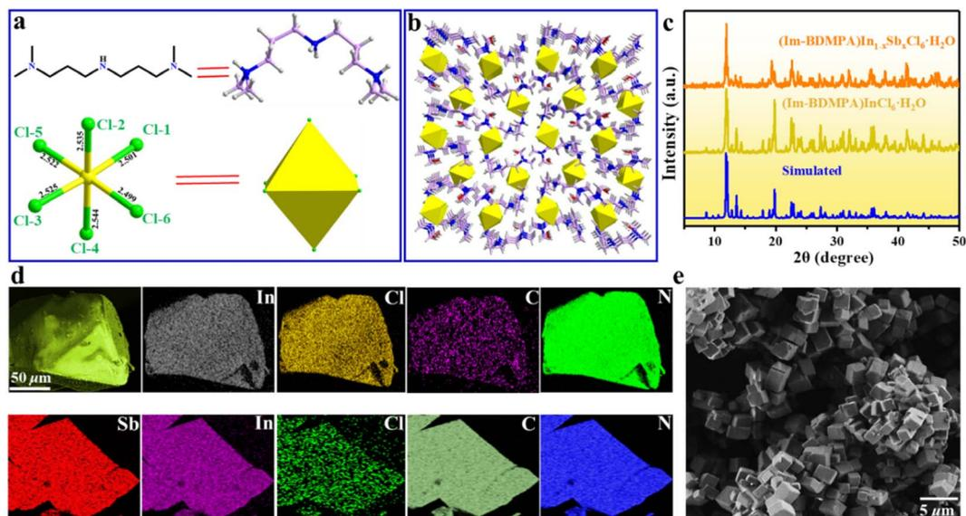
Fig. 1 Structural characterization of  $(\text{Im-BDMPA})\text{In}_{1-x}\text{Sb}_x\text{Cl}_6 \cdot \text{H}_2\text{O}$ : (a)  $(\text{Im-BDMPA})^{3+}$  cation and  $[\text{In/SbCl}_6]^{3-}$  octahedron; (b) packing structure of the OD structure viewed along the  $a$ -axis; (c) simulated and experimental PXRD patterns; (d) elemental mapping of SEM images; (e) SEM image of a microparticle.
