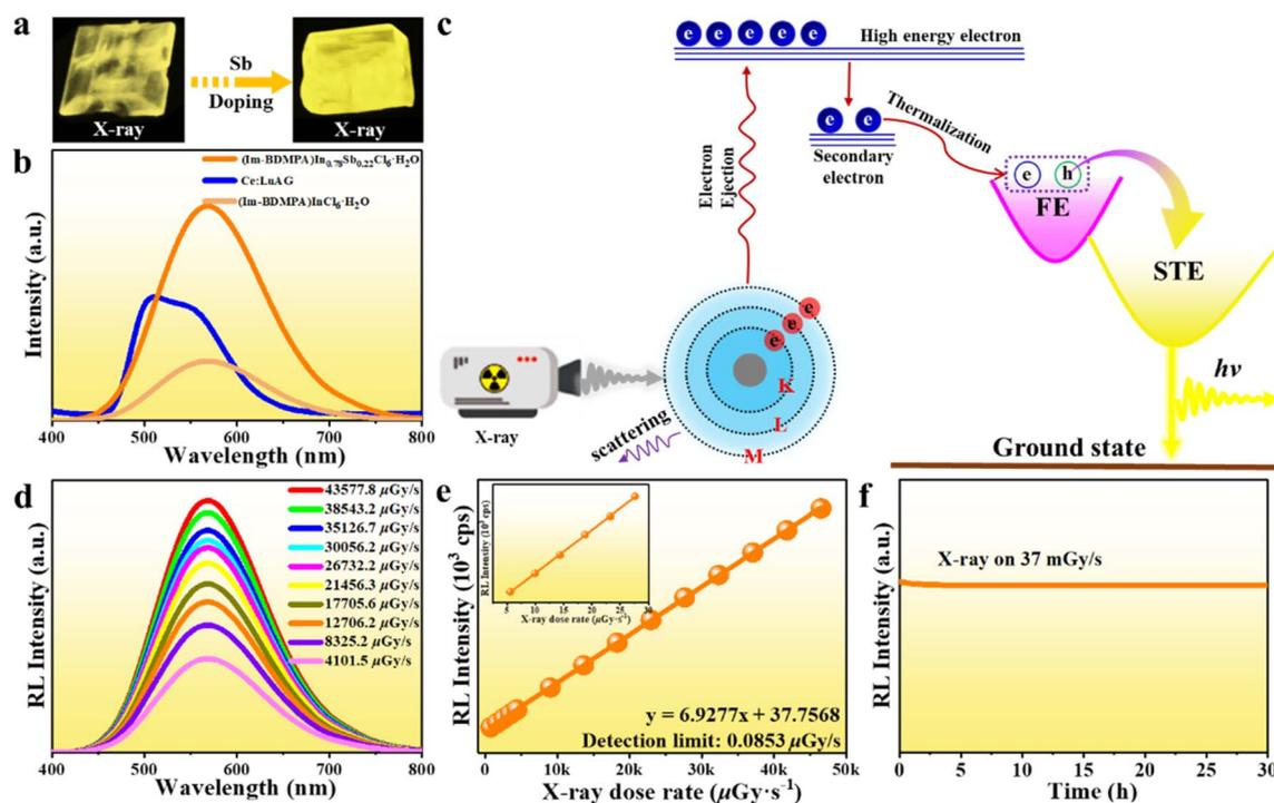
Fig. 5 X-ray scintillation performance of  $(\text{Im-BDMPA})\text{In}_{1-x}\text{Sb}_x\text{Cl}_6 \cdot \text{H}_2\text{O}$ : (a) photo images of bulk crystals under X-ray irradiation; (b) RL spectra under 30 kV X-ray excitation; (c) proposed radioluminescence mechanism; (d) X-ray dose rate dependent RL emission spectra; (e) linear dependence of RL emission intensity vs. X-ray dose rate; (f) monitored RL emission intensity under continuous X-ray irradiation.
