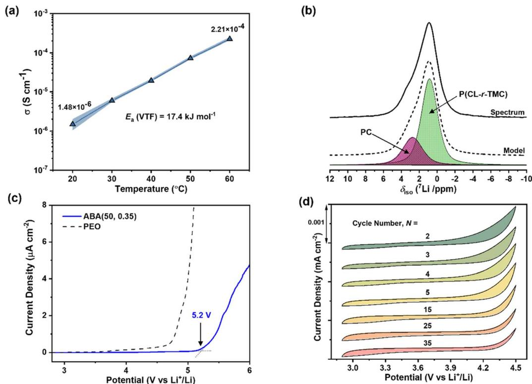
Fig. 3 (a) Temperature-dependence of ionic conductivity for ABA (50, 0.35)/17 wt% LiTFSI. (b) Solid-state  $^7\text{Li}$  NMR spectrum with peak deconvolution to PC and P(CL-*r*-TMC) phases. (c) Oxidative stability vs. Li metal and stainless-steel counter electrode measured by LSV at 60 °C, 0.1 mV s $^{-1}$  scan rate. (d) CV at 0.5 mV s $^{-1}$  scan rate recorded over 35 cycles.
