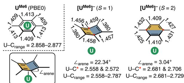
Fig. 7 A schematic of the optimised U–arene geometry in neutral  $[U^{Me6}]$ , and both intermediate-spin ( $S = 1$ ) and high-spin ( $S = 2$ )  $[U^{Me6}]^-$ , highlighting U–C and C–C bond lengths (Å), and the  $\angle_{arene}$  parameter.
