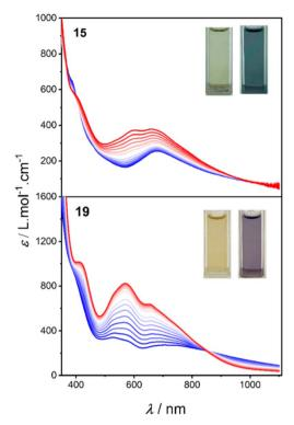
Fig. 5 Variable temperature electronic absorption spectra in MeCN for complexes 15 (273–333 K) and 19 (268–343 K). Figure insets are photographs of the low and high temperature solutions.
