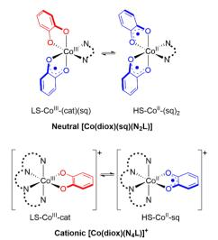
Fig. 1 Valence tautomeric interconversions for [Co(diox)(sq)(N<sub>2</sub>L)] and [Co(diox)(N<sub>4</sub>L)]<sup>+</sup> families of Co-dioxolene complexes.
