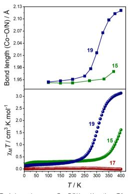
Fig. 4 (Top) change in average Co-O/N bond length vs. T for 15.BPh<sub>4</sub> (green squares) and 19.BPh<sub>4</sub> (blue squares); and (bottom) plot of  $\chi_{\rm M}T$  vs. T for the first heating of 15.BPh<sub>4</sub> (green spheres), 19.BPh<sub>4</sub> (blue spheres) and 17.BPh<sub>4</sub> (red spheres).
