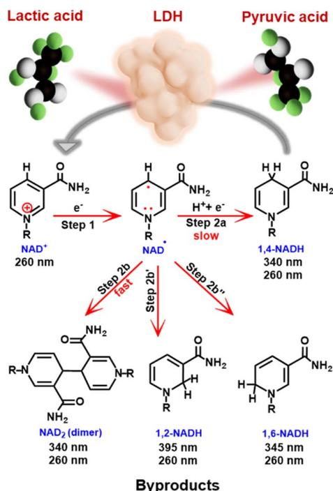
Scheme 1 Mechanism of electrochemical reduction of NAD<sup>+</sup>, possible products and wavelengths of observable UV absorption peaks for each product. Application of the enzymatically active 1,4-NADH for lactic acid formation is also illustrated.
