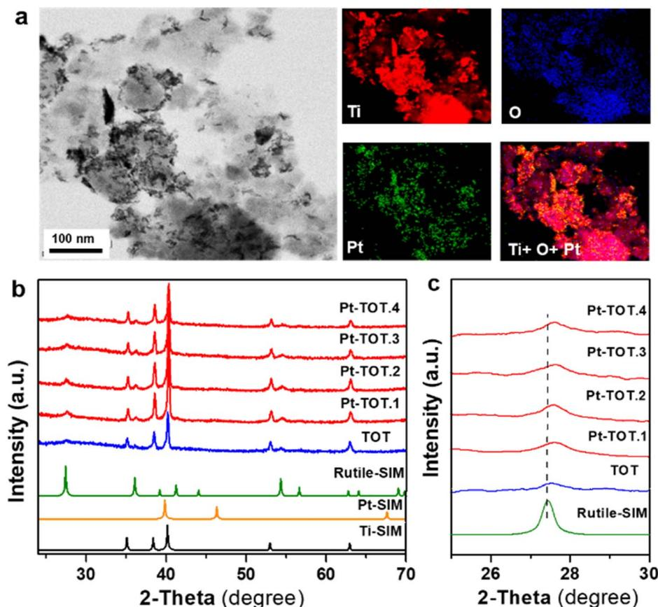
Fig. 1 (a) STEM and EDS elemental mapping of **Pt-TOT.2**, (b) XRD pattern, and (c) expanded XRD pattern from  $2\theta = 24$  to  $30^\circ$  of TOT and **Pt-TOTs** with different Pt content (the dashed line shows the diffraction peak position of rutile  $\text{TiO}_2$ ).
