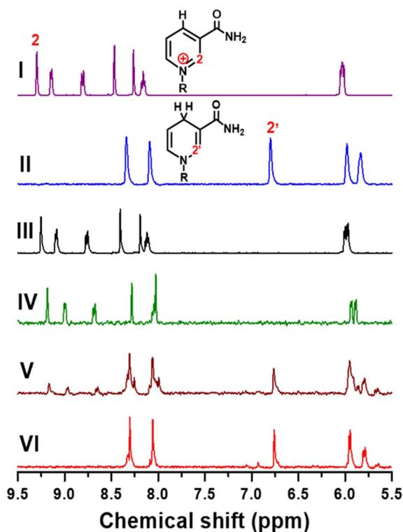
Fig. 3  $^1\text{H}$  NMR spectra of  $\text{NAD}^+$  (4 mM in 0.1 M  $\text{D}_2\text{O}$  phosphate buffer, pH 6) (I), 1,4-NADH (4 mM in 0.1 M  $\text{D}_2\text{O}$  phosphate buffer, pH 6) (II), products generated from 4 mM  $\text{NAD}^+$  in 0.1 M  $\text{D}_2\text{O}$  phosphate buffer with pH 5.8 at  $-0.8$  V vs. Ag/AgCl on TOT (III) for 2 h, Pt (IV) for 2 h, and **Pt-TOT.2** (V) for 2 h, and on **Pt-TOT.2** (VI) for 4 h.
