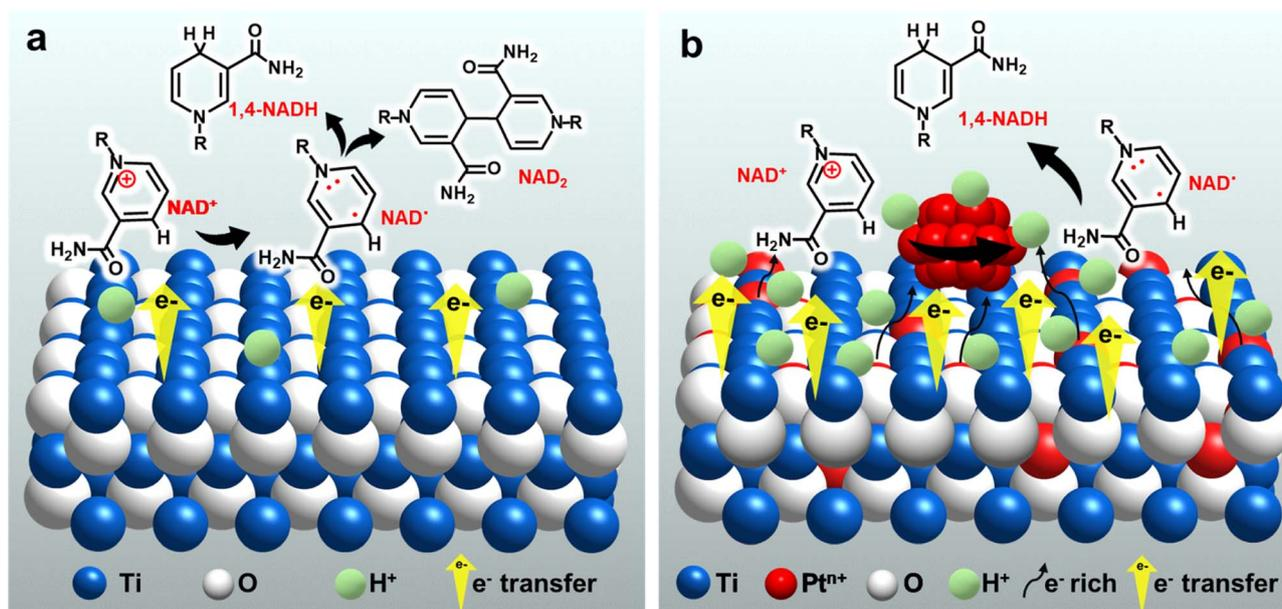
Scheme 2 Suggested strategy and mechanism for the electrochemical reduction of NAD<sup>+</sup> on (a) TOT and (b) Pt-TOTs.
