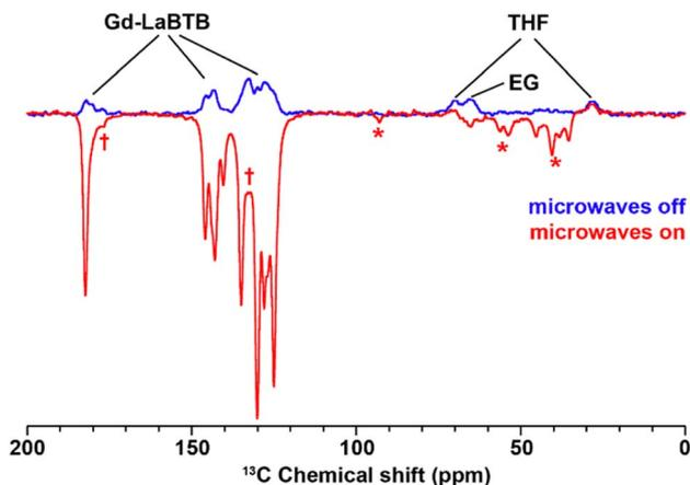
Fig. 8  $^{13}\text{C}$  MAS NMR spectra acquired for 23.5 mM Gd-LaBTB loaded with EG/THF at 100 K with (red) or without (blue) microwaves at the optimal field position (negative lobe in the  $^{13}\text{C}$  field-sweep profile shown in Fig. 5). Asterisks indicate spinning side bands. Daggers indicate new MOF resonances appearing upon introduction of EG/THF.
