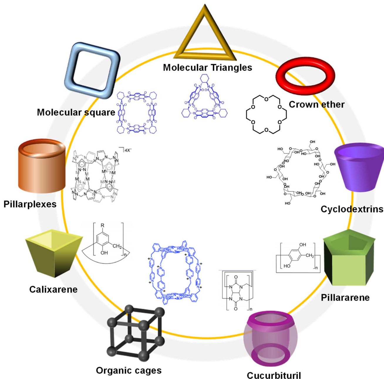
Fig. 1 Typical macrocycles with different spatial topological structure for the preparation of host–guest complex.
