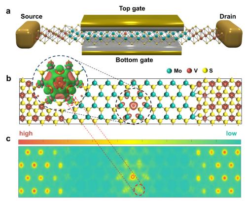
Fig. 2 Schematic diagram of a FET model with  $VS_2$  electrodes at both ends, V-MoS<sub>2</sub> channel in the middle ( $L_{ch}$  = 3.0 nm), and gate electrodes (EOT = 0.5 nm) on top and bottom (a). The real-space DOS at -0.2 eV (b) and corresponding 2D plot (c) are shown with zero source-drain bias applied. The inset in (b) represents the differential charge density at the V-doped site.
