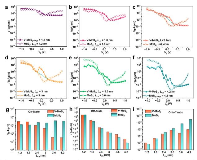
Fig. 3 (a)–(f) Transfer characteristics of MoS<sub>2</sub> (hollow circles) and V-MoS<sub>2</sub> (solid spheres) at  $L_{ch} = 1.2$  nm (a), 1.8 nm (b), 2.4 nm (c), 3.0 nm (d), 3.6 nm (e), and 4.2 nm (f), under a source bias of 0.2 V. Shown in (g-i) are the comparison of the on-state currents (g), off-state currents (h), and on/off ratios (i) between V-MoS<sub>2</sub> (orange) and MoS<sub>2</sub> (cyan) at different  $L_{ch}$
