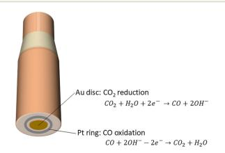
Fig. 3 Schematic illustration of rotating ring disc electrode. Electrocatalytic CO<sub>2</sub> reduction to CO takes place on Au disc electrode, and subsequently oxidation of CO into CO<sub>2</sub> occurs on Pt ring electrode.
