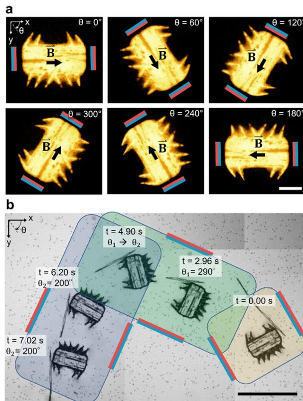
**Fig. 4** Magnetic manipulation of a soft polymeric microrobot. (a) Controlled rotational motion of a fluorescent microrobot in a glycerol/distilled water mixture (50/50 vol%). Scale bar, 100  $\mu\text{m}$ . In the stitched image sequence (b), the navigation of a microrobot along a 90-degree curved pathway using external magnetic field guidance and acoustic propulsion ( $f = 23.3 \text{ kHz}$ ,  $V_{\text{pp}} = 22.5 \text{ V}$ ) is shown. Scale bar, 500  $\mu\text{m}$ .
