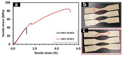
Stress-strain curves (a) of MEX 3D printed samples of 70/30/0 and 70/30/5 along with fractured tensile specimens ((b) 70/30/0; (c) 70/30/5).
