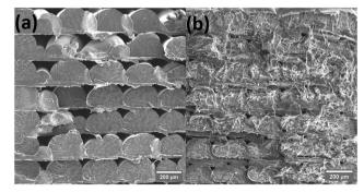
SEM images of fractured cross-sectional surfaces of MEX printed tensile specimens of PLA/PBAT ((a) 70/30/0) and PLA/PBAT/ECO ((b) 70/ 30/5).
