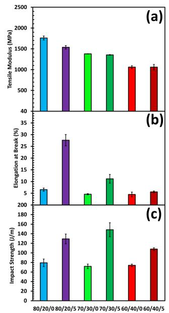
Fig. 5 Effect of ECO on the elongation at break (a), tensile modulus (b), and (c) the impact strength of PLA/PBAT blends.
