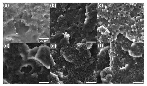
Fig. 2 SEM micrographs of fractured surfaces of PLA/PBAT ((a) 80/20, (b) 70/30, and (c) 60/40) and PLA/PBAT/ECO ((d) 80/20/5, (e) 70/30/5, and (f) 60/40) 40/5) blends. All scale bars are 20 μm.
