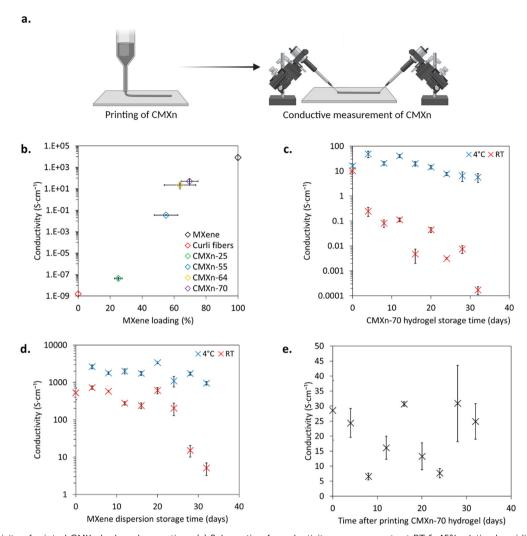
Fig. 5 Conductivity of printed CMXn hydrogels over time. (a) Schematic of conductivity measurements at RT & 45% relative humidity (RH) for printed CMXn hydrogels, followed by (b) conductivity measurements of CMXn hydrogels plotted as a function of their MXene load, (c) shelf life of CMXn-70 hydrogel at refrigerated (4 °C) and RT conditions, (d) shelf life of MXene dispersion at 4 °C and RT & (e) stability of printed CMXn-70 hydrogel.
