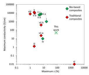
Fig. 6 Comparison of maximum ultimate strain (¿) and maximum conductivity achieved by other MXene composite films using different manufacturing techniques. Nomenclature and numerical values are shown in Table S1 (ESI†). Further mechanical properties and assembly techniques are shown in Table S2 (ESI†)
