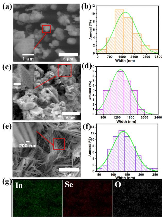
Fig. 4 Surface morphology and size distribution analysis of (a) and (b)  $\text{In}_2\text{S}_3$  nanostructures, (c) and (d)  $\text{In}_2\text{S}_{1.5}\text{Se}_{1.5}$  nanostructures and nanoplates, and (e) and (f)  $\text{In}_2\text{Se}_3$  nanofibers, and (g) EDS mapping of  $\text{In}_2\text{Se}_3$  nanofibers.
