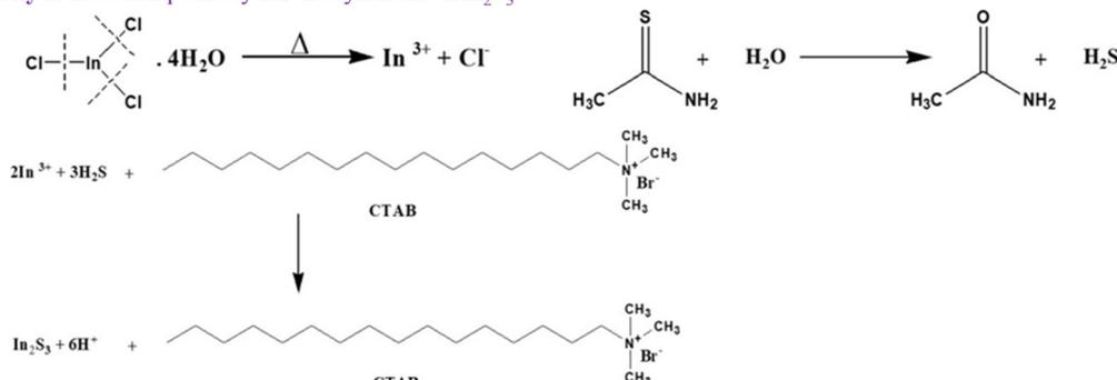
Fig. 1 The reaction pathway for the synthesis of  $\text{In}_2\text{S}_3$ ,  $\text{In}_2\text{Se}_3$  and  $\text{In}_2\text{S}_{1.5}\text{Se}_{1.5}$  nanostructures.
