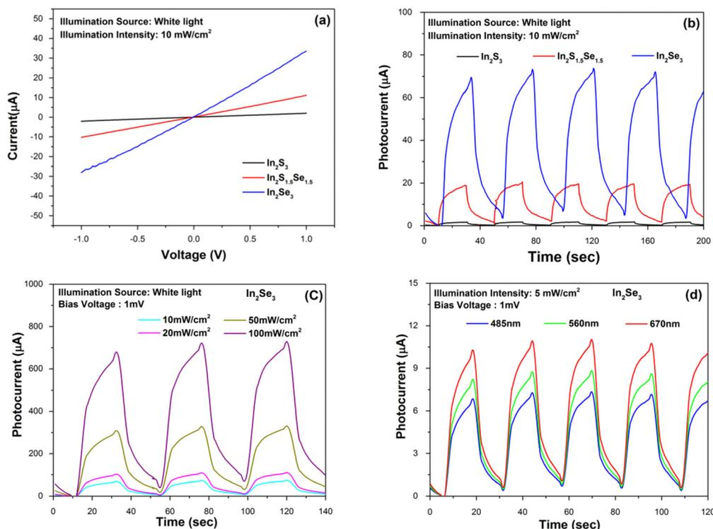
Fig. 5 The (a)  $I$ - $V$  characteristics, (b) pulse photoresponse of  $\text{In}_2\text{S}_3$ ,  $\text{In}_2\text{S}_{1.5}\text{Se}_{1.5}$ , and  $\text{In}_2\text{Se}_3$  nanostructures, (c) pulse photoresponse of  $\text{In}_2\text{Se}_3$  nanofibers at different illumination, and (d) pulse photoresponse of  $\text{In}_2\text{Se}_3$  nanofibers at different intensity.
