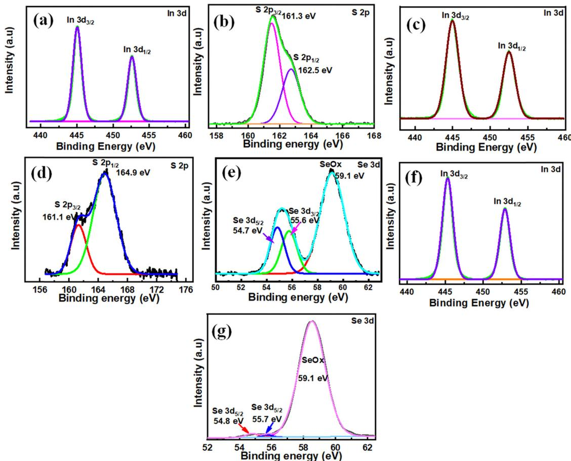
Fig. 2 (a) and (b) The core level spectra of indium (In 3d) and sulfur (S 2p) in  $\text{In}_2\text{S}_3$  nanostructures. (c)–(e) The core level spectra of indium (In 3d), sulfur (S 2p), and selenium (Se 3d) in  $\text{In}_2\text{S}_{1.5}\text{Se}_{1.5}$  nanostructures. (f) and (g) The core level spectra of indium (In 3d) and selenium (Se 3d) in  $\text{In}_2\text{Se}_3$  nanostructures.
