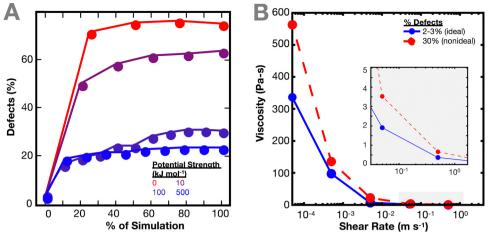
Fig. 3 Effect of defects on viscosity of polymer network. (A) Defects in network based on individual crosslinks for  $10^{-9}$  fs<sup>-1</sup> engineering strain rate across different interaction potentials. The defects increase over simulation time. (B) Comparison of viscosity of network with 2–3% initial defects *versus* ~30% initial defects for an interaction potential of 100 kJ mol<sup>-1</sup>.
