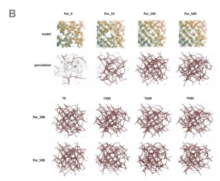
Fig. 4 Percolation was assessed within each polymer network at multiple time steps under deformation. (A) Percolation was measured by comparing the number of possible paths between distant points on the network's periphery to the number of viable shortest walks through the network between those points. (B) Each network demonstrated different degrees of connectivity, and the number and form of viable paths through the network changed under deformation
