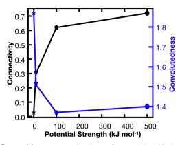
**Fig. 5** Connectivity vs. convolutedness for models with interaction potentials of 0, 10, 100, 500 kJ  $\text{mol}^{-1}$ . As the interaction potential increases, the connectivity of the network goes up, while the convolutedness goes down. This implies that a stronger potential holds the network together more robustly.
