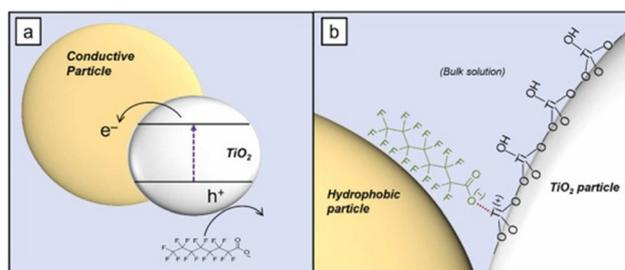
Fig. 10 Schematic depicting the hypothesized interaction between the hydrophobic graphene support and the  $\text{TiO}_2$  semiconductor for PFOA oxidation.<sup>60</sup>
