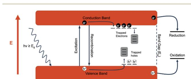
**Fig. 8** Diagram depicting the absorbance of a photon in a semiconducting material, resulting in the generation of an exciton. The generated electron exists within the conduction band, whereas the hole exists within the valence band. By 'trapping' either the conduction band electron or valence hole, the lifetime of the generated exciton pair can be elongated. Generated electrons undergo reduction and generated holes undergo oxidation. This figure was created by the authors.
