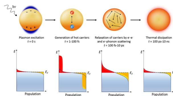
Fig. 4 Plasmon induced hot hole generation resulting in thermal dissipation with time frames.<sup>40</sup>
