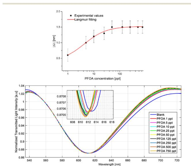
**Fig. 6** Test results by Pitruzzella *et al.* for their MIP sensor within a simulated seawater matrix. The data readings (top) combined with the noted change in the observed wavelength with increasing concentration (bottom) indicate that the sensitivity of the sensor decreases with higher concentrations.
