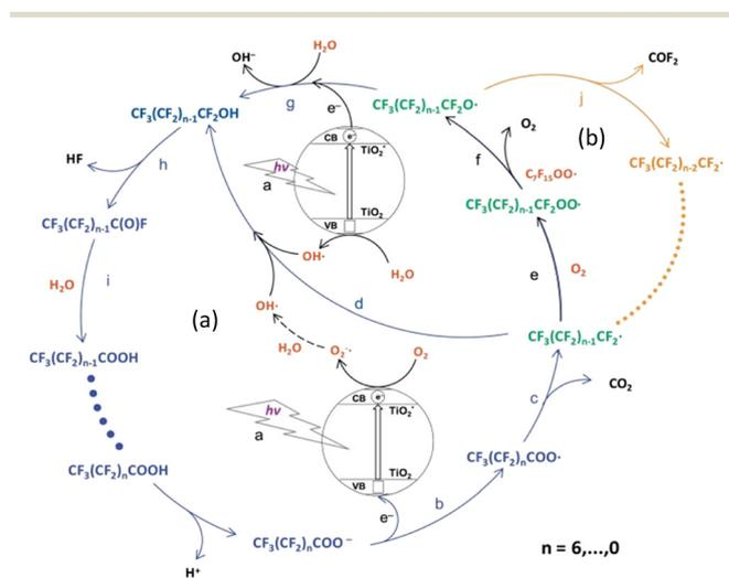
**Fig. 9** Diagram of potential PFCA degradation pathways *via* radical generation. Photo-redox pathway (blue arrows (a)) and  $\beta$ -scission pathway (orange arrows (b)).<sup>52</sup> This image has been modified from its original publication.
