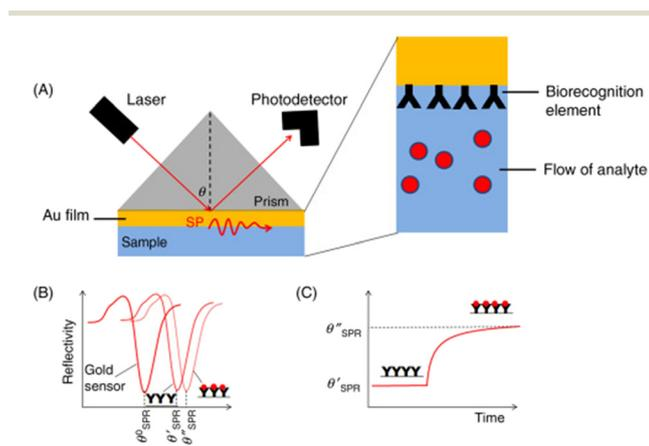
**Fig. 5** Example of SPR sensing technology. As the analyte binds onto the sensor's surface (a), a shift in the incident angle for SPR is noted (b), indicating that the analyte is present. As more analyte binds, the change in angle levels off (c).<sup>37</sup> This figure has been modified from its original publication.
