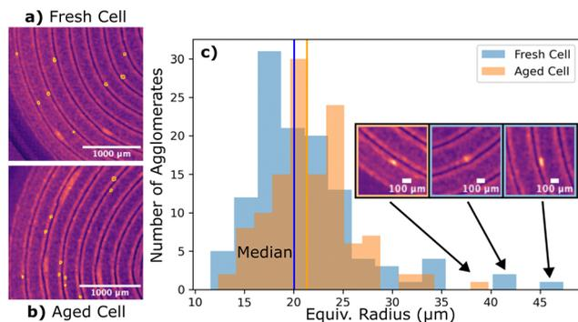
**Fig. 6** Size and shape of small silicon agglomerates defects. Visualization of small agglomerates in fresh (a) and (b) aged cells using the SAXS-CT integrated intensities. Agglomerates appear as bright spots of excess SAXS intensity and are marked by orange circles. (c) Histogram of the agglomerate size distribution, with inserts showing the largest agglomerates locations and shapes.
