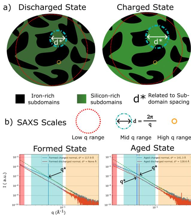
Fig. 4 Concept of SAXS-Analysis of nanostructured material. (a) Shows a stylized depiction of the nanostructure of the Si– $\text{FeSi}_2$  composite material. (b) Shows two averaged raw SAXS profiles extracted in regular areas for the formed and aged cells respectively, with one curve for the charged state and one curve for the discharged state to highlight the differences in shape caused by the expanding nanostructure.
