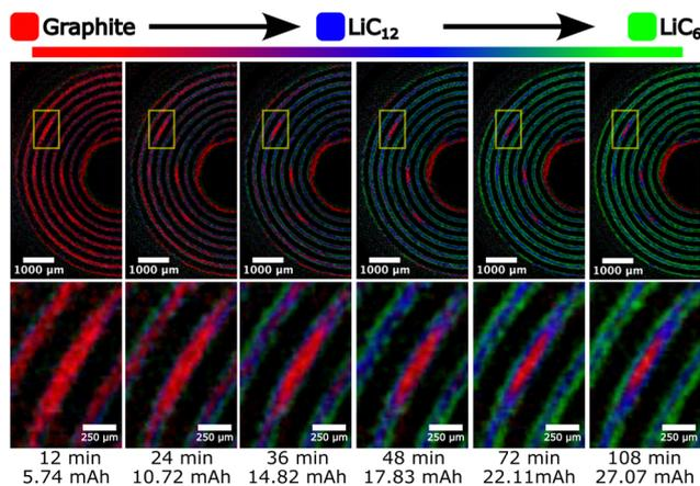
Fig. 5 Dynamics of graphite lithiation in large defective zones by operando WAXS-CT.  $\text{LiC}_6$  is depicted as green,  $\text{LiC}_{12}$  as blue, and poorly lithiated graphite ( $\text{Li}_x\text{C}_6$  with  $x < 0.2$ ) as red. Top row: An overview of the aged cell. Bottom row: Zoom on the selected bent area. An elliptically shaped area of graphite can be observed, which slowly shrinks during the charge, lagging behind the rest of the cell.
