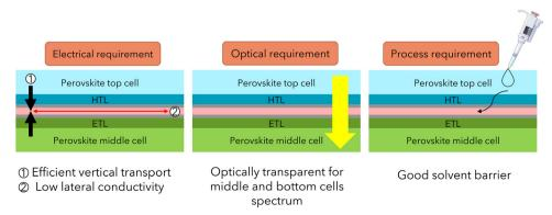
Fig. 15 Schematic of relevant electrical, optical and processing requirements for the monolithical connection of perovskite subcells.
