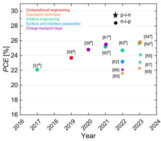
PCE evolution of FAPblz solar cells in p-i-n and n-i-p configuration discussed in this review for different strategies that resulted in efficient solar cells and improved stability (red: compositional engineering, orange: deposition technique, green: additive engineering, blue: surface and interface passivation and purple: charge transport layer). Data for n-i-p configuration are taken from ref. 54 and 57-64 and for p-i-n configuration from ref. 55 and 65-68. Certified values are marked with #
