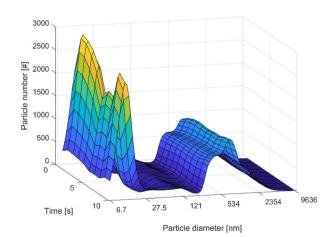
Fig. 8 Bimodal size distribution. Data correspond to the first ten seconds during run-in.
