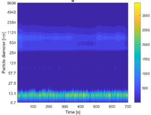
Fig. 7 Particle size distribution of the phases in Fig. 6. (a) Run-in, and (b) steady state. Note the bi-modal size distribution for both phases.
