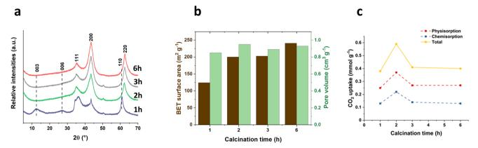
Fig. 4 (a) XRD of 400-X-100 samples. (b) BET surface area and pore volume of 400-X-100 samples, and (c) CO<sub>2</sub> adsorption for 400-X-100 samples at 40 °C and 100 kPa
