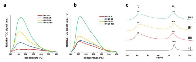
Fig. 2 (a) NH<sub>3</sub> TPD, (b) CO<sub>2</sub> TPD of 400-2 h-X samples and (c) <sup>27</sup>Al DPMAS ssNMR of (i) Mg<sub>2</sub>Al LDH, (ii) 400-2 h-5, (iii) 400-2 h-50 and (iv) 400-2 h-100.
