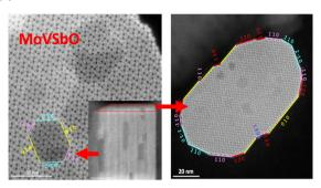
Study of super-efficient defective MoVSbO catalysts used for ethane oxidative dehydrogenation by HAADF-STEM and of their thermal evolution by environmental electron microscopy and tomography
