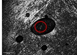
Fig. 5 Polarised-light microscope images of CAOC at 15 °C, showing birefringence and a Maltese cross pattern (red circle) indicative of a lamellar liquid crystalline phase. The images are taken at different points of the same sample slide with  $4\times$  magnification (left) and  $10\times$  magnification (right).
