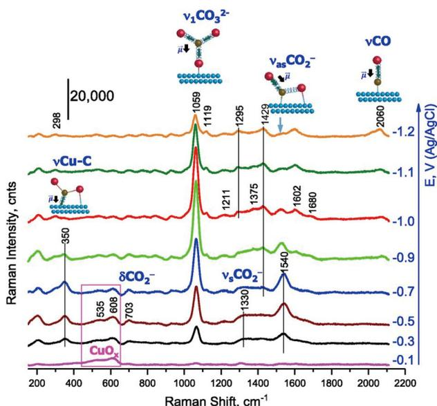
Fig. 2 *Operando* SERS of the rough Cu surface in CO<sub>2</sub>-saturated 0.1 mol dm<sup>-3</sup> NaHCO<sub>3</sub> (pH 6.8). Spectra were measured in the cathodic direction from -0.1 V. Adapted with permission from ref. 44. Copyright 2018 National Academy of Sciences.
