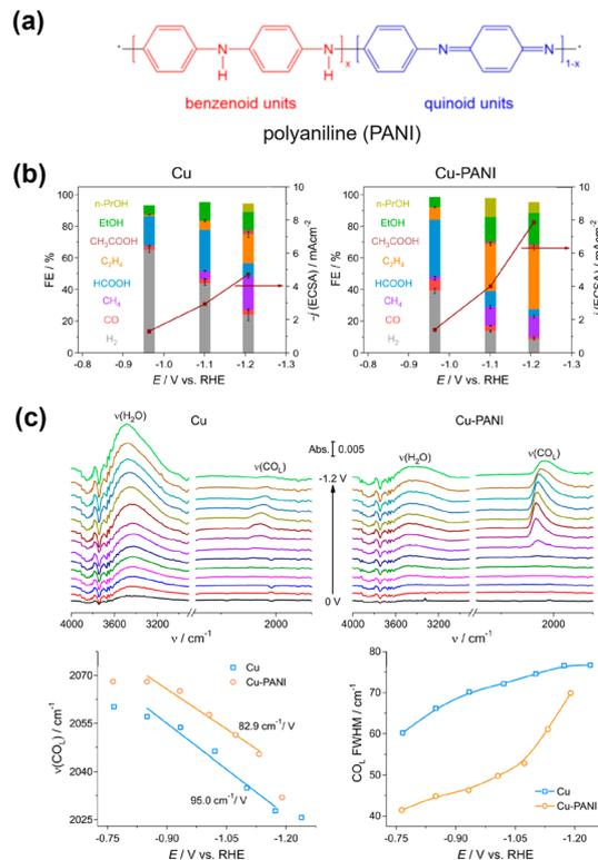
**Fig. 11** (a) Structure of PANI. (b) Modification effect on the  $CO_2RR$ . (c) (top) *In situ* ATR-SEIRAS spectra of the  $CO_2RR$  on the Cu and Cu-PANI electrodes, respectively, in  $CO_2$  saturated 0.1 M  $KHCO_3$ . (bottom) Stark effects of the linearly adsorbed CO ( $CO_L$ ) and full width at half-maximum (FWHM) of  $CO_L$  signals. Reproduced with permission from ref. 78. Copyright 2020 American Chemical Society.
