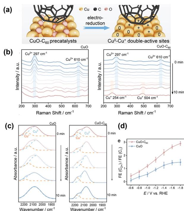
**Fig. 13** (a) Schematic illustration of the electroreduction of CuO-C<sub>60</sub> precatalysts. (b) *In situ* Raman spectra of CuO and CuO-C<sub>60</sub> precatalysts at a reduction potential of -0.4 V versus RHE. (c) *In situ* ATR-FTIR spectra under continuous CO<sub>2</sub> flow over CuO and CuO-C<sub>60</sub>. (d) The Faraday efficiency ratios of C<sub>2+</sub> to C<sub>1</sub> products from the CO<sub>2</sub>RR. Reproduced with permission from ref. 82. Copyright 2023 Wiley.
