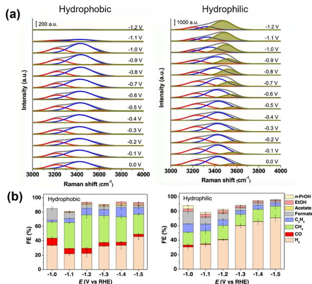
**Fig. 8** (a) *In situ* Raman spectra of the O-H stretching mode of interfacial water molecules with (hydrophobic) and without (hydrophilic) modification with 1-octadecanethiol. Peaks are deconvoluted. (b) Effect of modification on CO<sub>2</sub>RR selectivity. Reproduced with permission from ref. 68. Copyright 2021 American Chemical Society.
