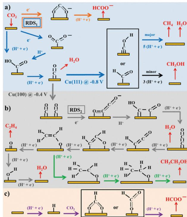
Fig. 1 Schemes of the possible reaction pathways of the CO<sub>2</sub>RR on transition metals: (a) pathway from CO<sub>2</sub> to CO, CH<sub>4</sub>, CH<sub>3</sub>OH, and formate, (b) pathways from CO<sub>2</sub> to ethylene and ethanol, and (c) pathway of CO<sub>2</sub> insertion into a metal–H bond yielding formate. Adapted with permission from ref. 19. Copyright 2015 American Chemical Society.
