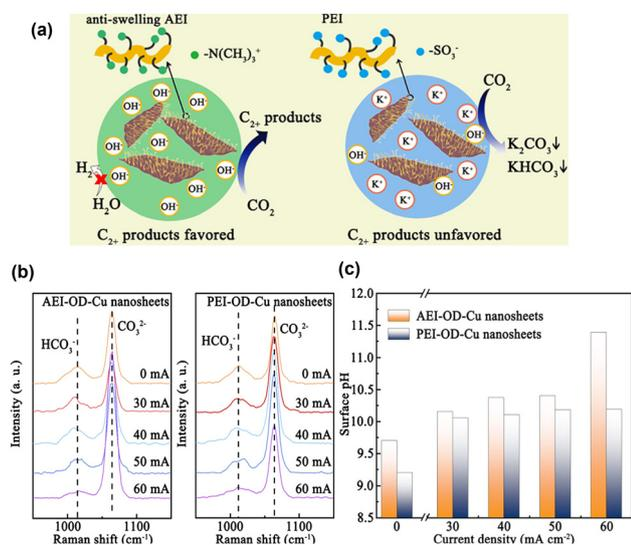
**Fig. 12** (a) Schematic illustration of CO<sub>2</sub>-to-C<sub>2+</sub> activity and selectivity through local environment construction. (b) *In situ* Raman spectra obtained from the AEI-OD-Cu and PEI-OD-Cu nanosheets. (c) pH values calculated from the *in situ* Raman spectra. Reproduced with permission from ref. 80. Copyright 2022 American Chemical Society.
