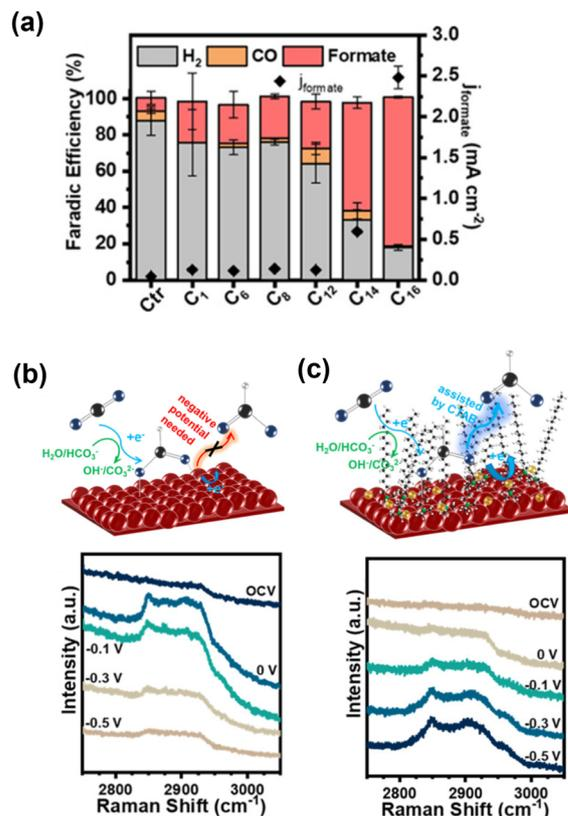
Fig. 10 (a) Dependence of the electrocatalytic CO<sub>2</sub> reduction performance of Cu on the straight-chain alkyl group R of the NR(CH<sub>3</sub>)<sub>3</sub>Br additive. (b) and (c) *In situ* Raman spectra of Cu and Cu-CTAB in CO<sub>2</sub>-saturated 0.5 M KHCO<sub>3</sub> under applied potentials, with the schematic illustration of formate formation. Reproduced with permission from ref. 73. Copyright 2020 American Chemical Society.
