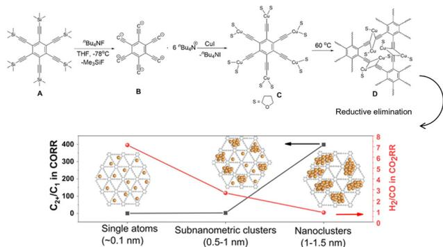
Fig. 15 Schematic illustration of the synthesis of the Cu/graphdiyne scaffold and the size effect of Cu(0) catalysts on CO<sub>2</sub>RR selectivity. Reproduced with permission from ref. 91. Copyright 2022 Wiley.
