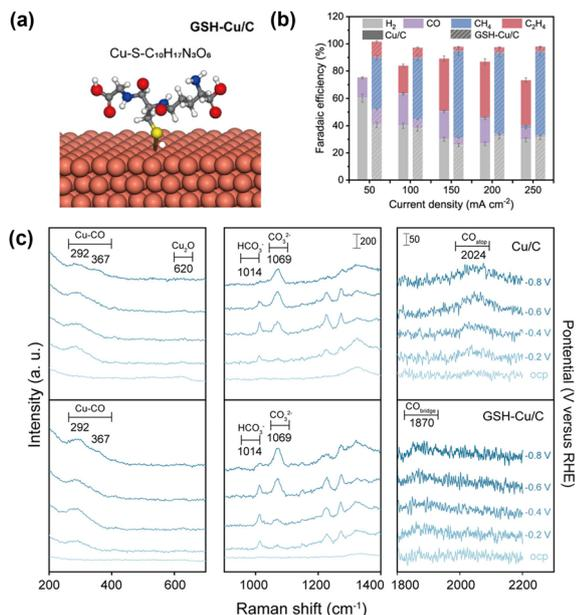
**Fig. 7** (a) Structure of modified Cu with glutathione (GSH). (b) Effect of GSH modification on the CO<sub>2</sub>RR product. (c) *Operando* Raman spectra for Cu/C and GSH-Cu/C in the potential range from the OCP to  $-0.8$  V vs. RHE. Reproduced with permission from ref. 67. Copyright 2022 American Chemical Society.
