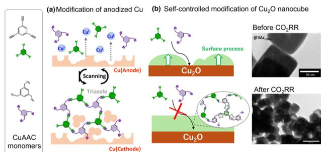
Fig. 16 Schematic illustration of two CuAAC modifications: on anodized Cu (a) and on Cu<sub>2</sub>O nanocubes, with TEM images of structural transformation upon the CO<sub>2</sub>RR (b). Reproduced with permission from ref. 93 and 94. Copyright 2022 Wiley.
