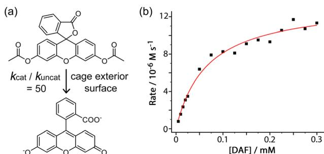
Fig. 3 (a)  $\text{H}^{\text{W}}$ -catalysed hydrolysis of diacetyl fluorescein; (b) dependence of the reaction rate on substrate concentration, fitted to a Michaelis–Menten reaction model to extract an association constant for the interaction between substrate and cage exterior surface (see main text).
