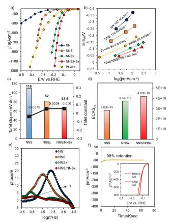
Fig. 4 (a) HER SCV curves with 100% iR compensation; (b) Tafel plots derived from SCV (catalytic turn-over region) for NN, NNS, NNS, and NNS/ NNSx; comparative bar diagram showing; (c) Tafel slope and Tafel constant; (d) ECAS<sub>Ni</sub> for NNS, NNS<sub>x</sub> and NNS/NNS<sub>x</sub>; (e) Bode-phase angle plot with time constant and (f) HER stability curve for NNS/NNS<sub>x</sub> with the inset showing before and after activity results.
