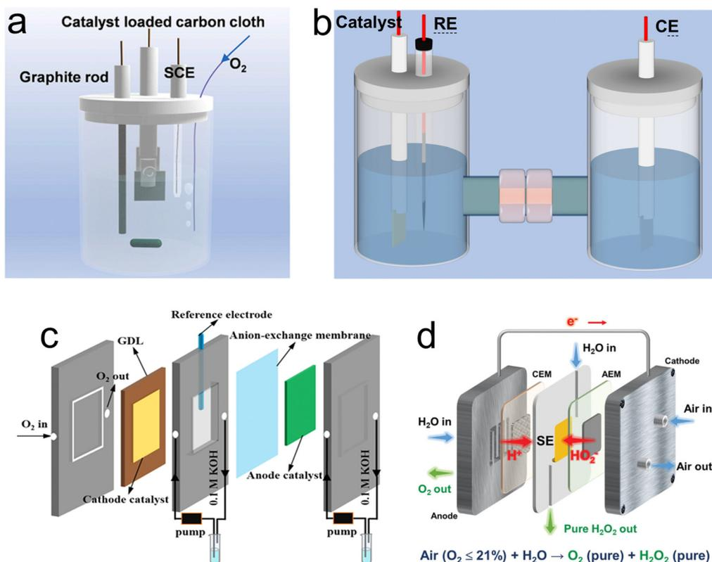
Fig. 5 Different types of setups for H<sub>2</sub>O<sub>2</sub> production. (a) One-pot setup. Reproduced from ref. 11. Copyright (2022) Elsevier. (b) H-cell. (c) Illustration of the flow cell setup. Reproduced from ref. 17. Copyright (2021) Wiley-VCH GmbH. (d) solid-electrolyte (SE) cell system. Reproduced from ref. 78. Copyright (2023) Wiley-VCH GmbH.
